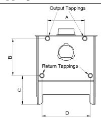
Freestanding boiler tapping measurements. Rear View example shown. Not to scale.
