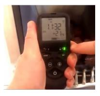
Hold the handset as shown, wrapping your hand around the handset touching both sides. In a second or less the green unlock light will illuminate, allowing the buttons to work when pushed. (NOTE: If the green light is not a constant green or not lit at all the buttons will not be operable).
