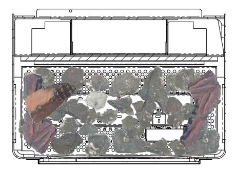
Position Log 3 (Inverted in position to log 2, as shown).
