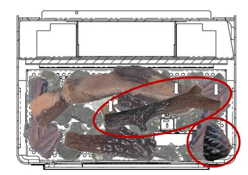
Position Log 7 as shown above. Note, this log sits on top of Log 6, Log 5 & Log 3 as shown with the arrows.
