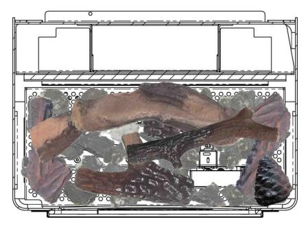
Position Log 7 as shown above. Note, this log sits on top of Log 6, Log 5 & Log 3 as shown.
