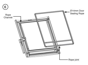
Remove the old rope and scrape old glue from the locating groove.
