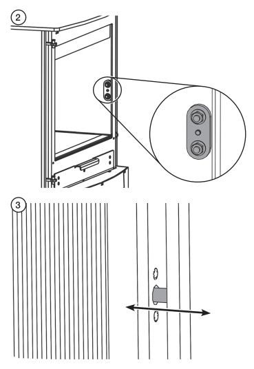
Fully tighten the nuts to secure the Catch.
