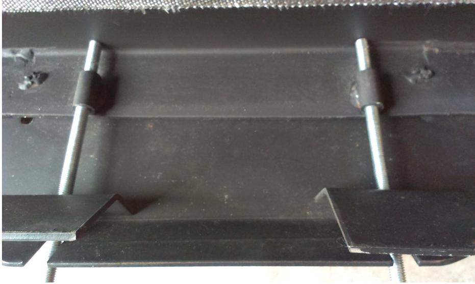
Slide the head brackets over the threaded bar and tighten with the 8mm nuts provided. Excess threaded bar should be trimmed to allow for sweeping.
