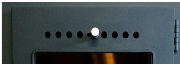
The primary air control knob, at the bottom of the Fire Door, should be set to closed (left) position as wood does not need air from below to burn effectively.
