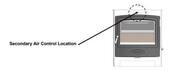
The control has an internal sliding plate with slots, housed inside the body of the appliance and is located centrally above the fire door assembly, when looking at the front of the appliance.
