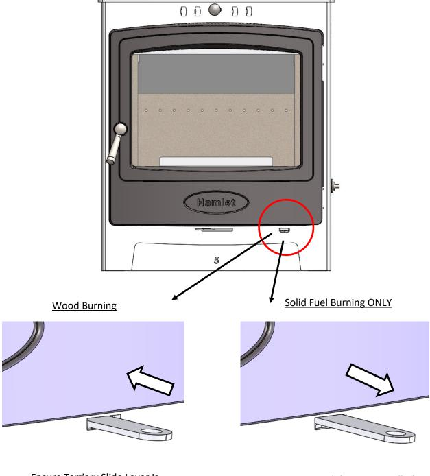
Ensure Tertiary Slide Lever Is Pushed Fully In (Wood Burning)
