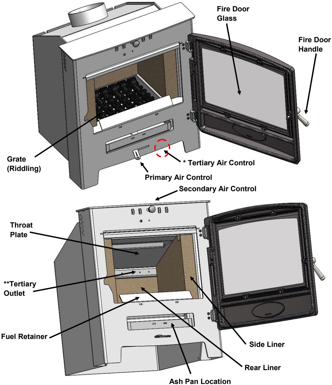
NOTE—\* 5kW Version Only—\*\* Integrated Into Rear Liner, 5kW Version Only
