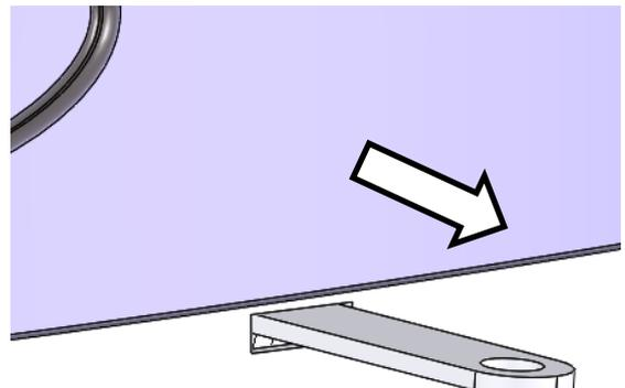
Ensure Tertiary Slide Lever Is Pulled Fully Outwards (Solid Fuel Burning)
