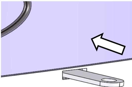
Ensure Tertiary Slide Lever Is Pushed Fully In (Wood Burning)
