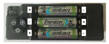
The remote display handset also has batteries as shown below. Again, remove the rear cover and replace the batteries (2 No. AA/1.5V LR6), observing the correct position as shown.
