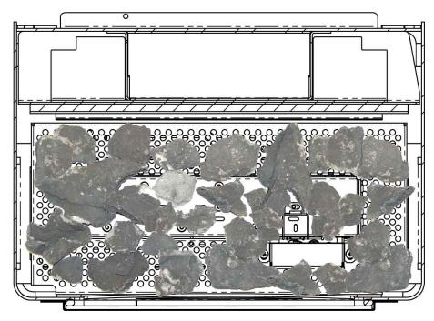
Scatter the bag of embers, evenly over the grate and burner, as shown above, ensuring the pilot and pilot shield are left clear from embers as indicated.
