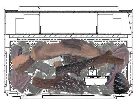
Position Log 7 as shown above. Note, this log sits on top of Log 6, Log 5 & Log 3 as shown.
