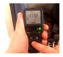
Press and hold in the power symbol button and release immediately as soon as the word pilot appears at the bottom left of the display (After about 1-2 seconds).
