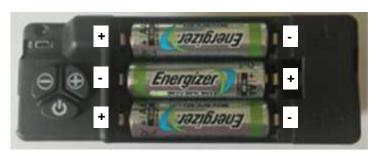
The remote control handset (RC) also has batteries as shown below. Again, remove the rear cover and replace the batteries (2 No. AA/1.5V LR6), observing the correct position as shown.
